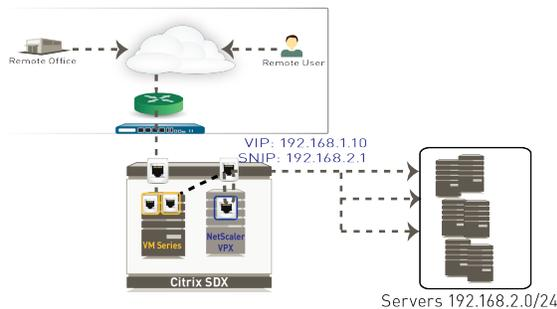
**Figure 7: Topology after adding the VM-Series firewall**
