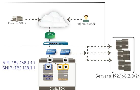
**Figure 5: Topology After Adding the VM-Series Firewall**
