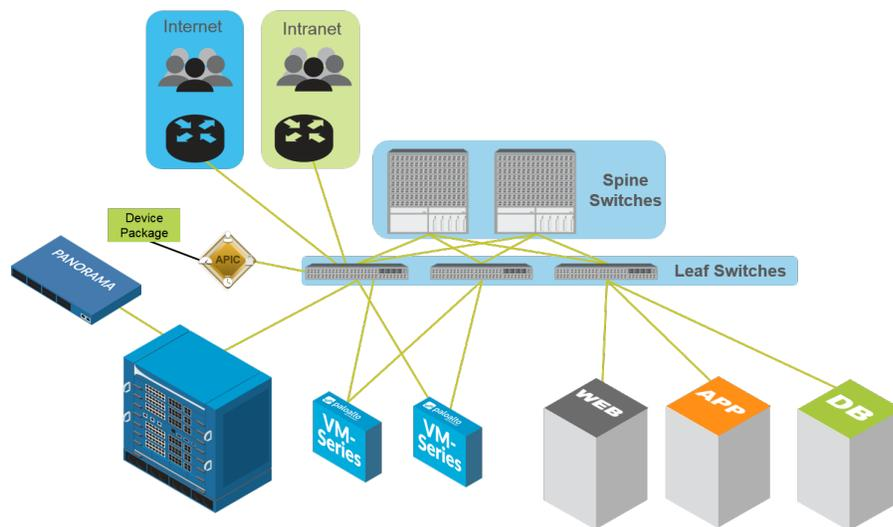
After the firewall services have been deployed, traffic now flows logically as shown below. Traffic to and from the end users and each tier in the application regardless of where or how each entity is physically connected to the network.
