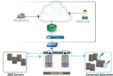
**Figure 8: Topology Before Adding the VM-Series Firewall**
