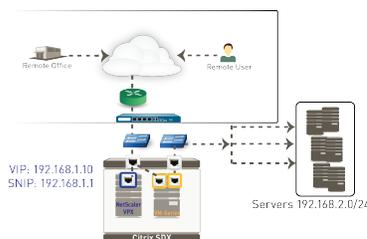
**Figure 2: Topology After Adding the VM-Series Firewall with L2 or Virtual Wire Interfaces**
