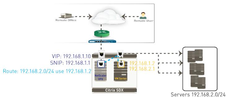
**Figure 4: Topology After Adding the VM-Series Firewall**
