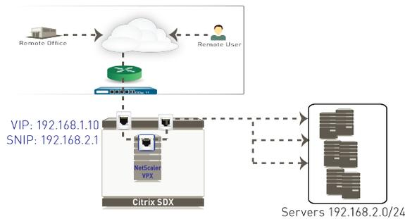
**Figure 6: Topology Before Adding the VM-Series Firewall**
