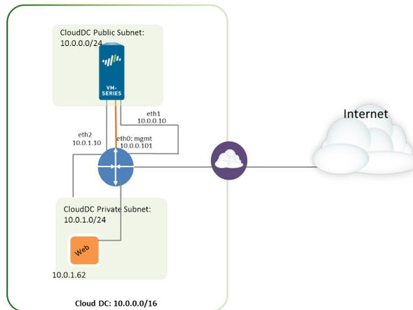
The following image depicts the logical flow of traffic to/from the web server to the internet. Traffic to/from the web server is sent to the data interface of the VM-Series firewall that is attached to the private subnet. The firewall applies policy and processes incoming/outgoing traffic from/to the internet gateway of the VPC. The image also shows the security groups to which the data interfaces are attached.
