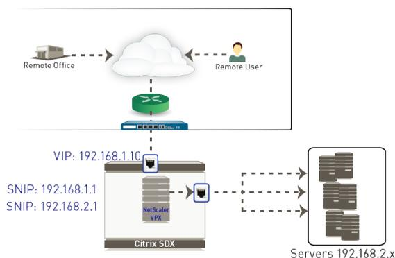
**Figure 3: Topology Before Adding the VM-Series Firewall**
