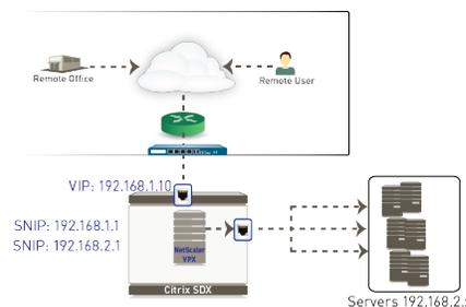
**Figure 1: Topology After Adding the VM-Series Firewall with L3 Interfaces**
